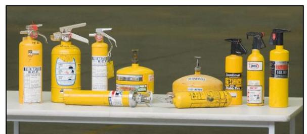
\*Halon numbers are designed for convenient and quick reference. The first digit of the number represents the number of carbon atoms in the compound molecule; the second digit, the number of fluorine atoms; the third digit, the number of chlorine atoms; the fourth digit, the number of bromine atoms; the fifth digit; the number of iodine atoms
